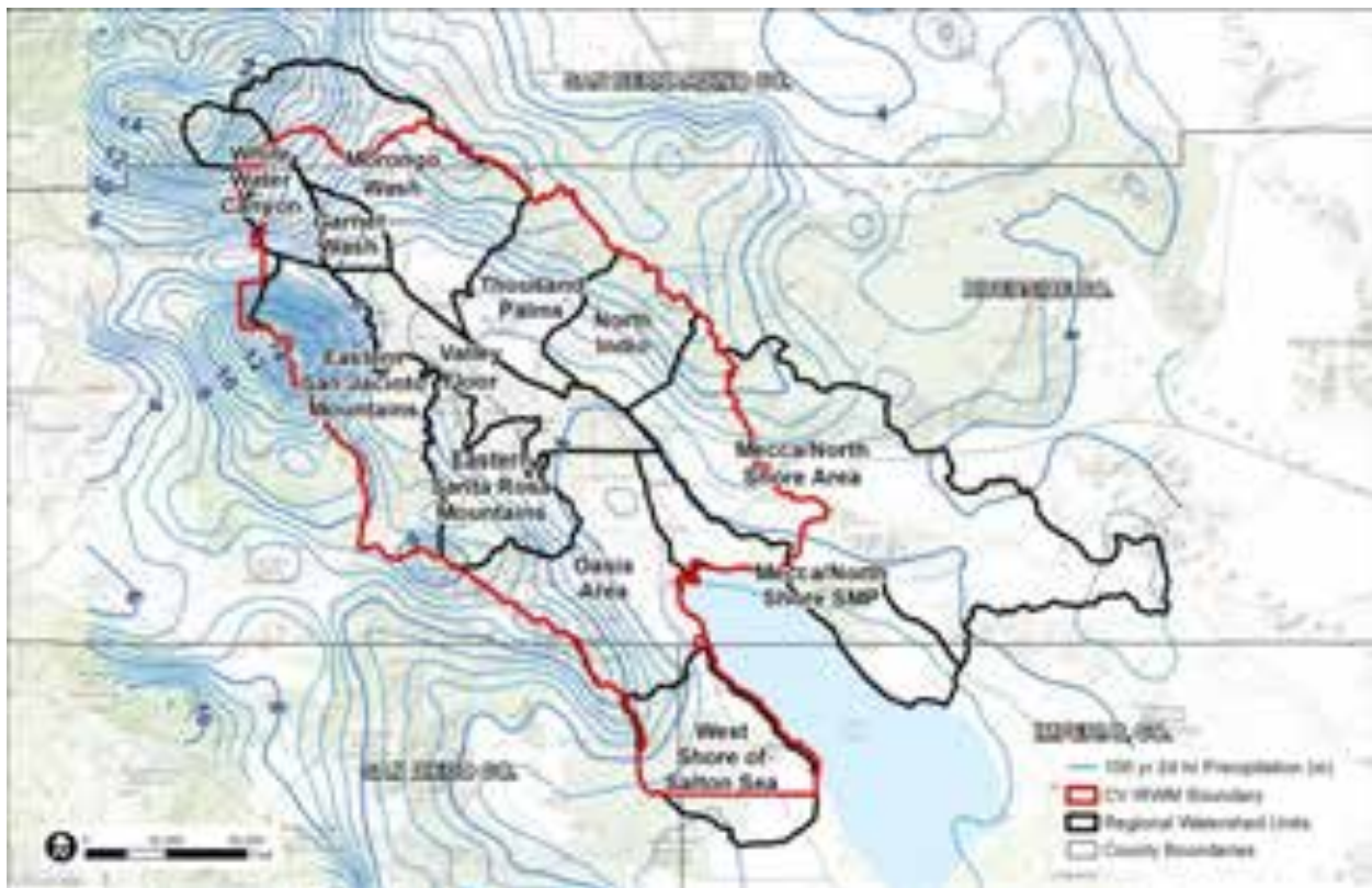
Figure 4-14: Coachella Valley 100-year 24-hour precipitation in inches variation illustrating lines of constant rainfall (isoplethials)
